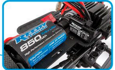
Reedy Power water-resistant speed control, 380 motor, servo and 850mah Li-Ion battery
