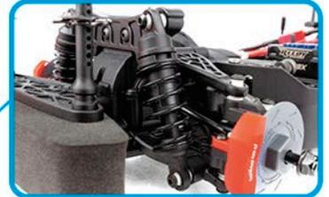
Coil-over shock absorbers smooth out the bumps when ripping around the rally course
