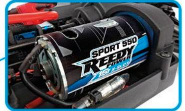
The Reedy 550 15-turn, 3-slot motor provides plenty of torque and tire-ripping speed
