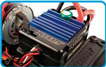
Controlling speed and power is the Reedy SC500X programmable brushed ESC (program card sold separately) with T-plug connector
