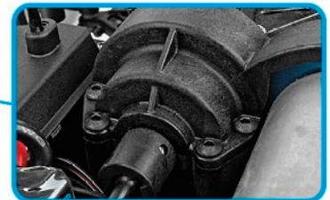
A sealed center driveline keeps dirt and debris out for smooth and reliable power delivery
