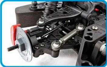
For better handling, A-arm front and rear independent suspension keeps the Apex2 chassis under control during the wildest of driving conditions
