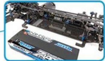
New battery mounting system for greater adjustability
