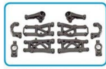
Ultra-lightweight carbon composite suspension components
