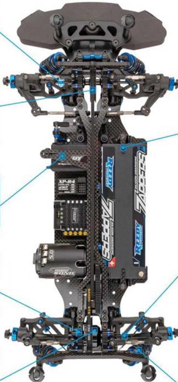
Ultra-lightweight carbon composite suspension components
